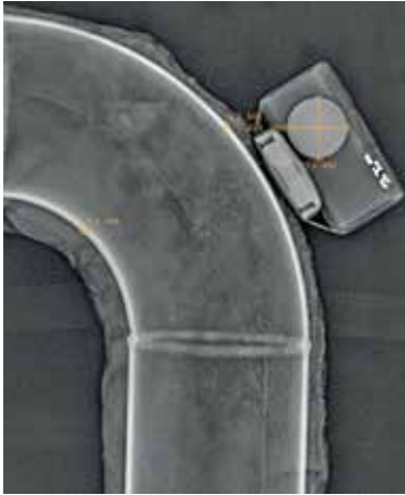
Wall Thickness Measurements
